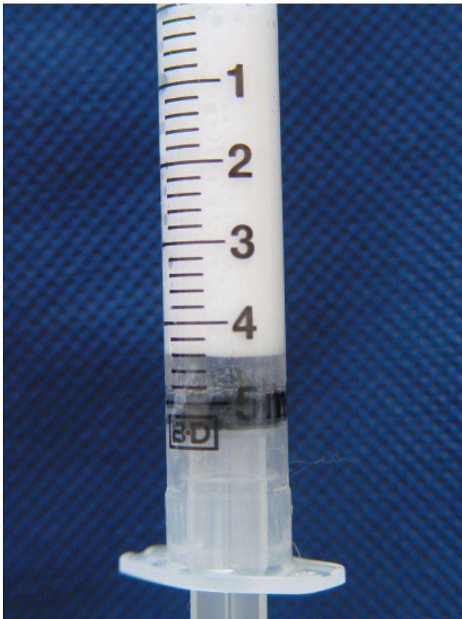
Figure 2. Measuring foam stability. With the timer started at the creation of the foam, the timer was stopped when the bottom of the fluid meniscus reached a level of 0.5 mL of solution (exactly half of the original 1.0 mL).
